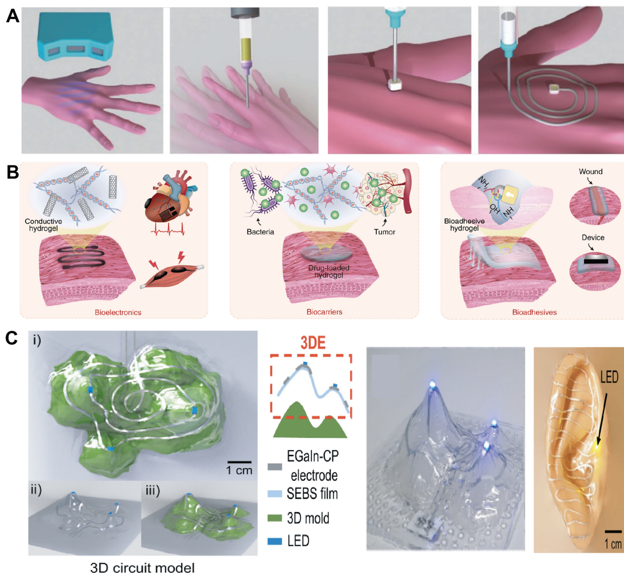
Figure 6. 3D conformal fabrication strategies for bioelectronics. (A) Adaptive 3D printing [205] . Copyright © 2018, WILEY-VCH Verlag GmbH & Co. KGaA; (B) Image-guided in vivo sound printing in deep tissues [206] . Copyright © 2025, the American Association for the Advancement of Science; (C) Conformal fabrication of 3D circuits on complex curvilinear surfaces [215] . Copyright © 2021, the American Association for the Advancement of Science. EGaIn-CP: eutectic gallium–indium with copper particles; SEBS: styrene–ethylene–butylene–styrene; LED: light-emitting diode.
