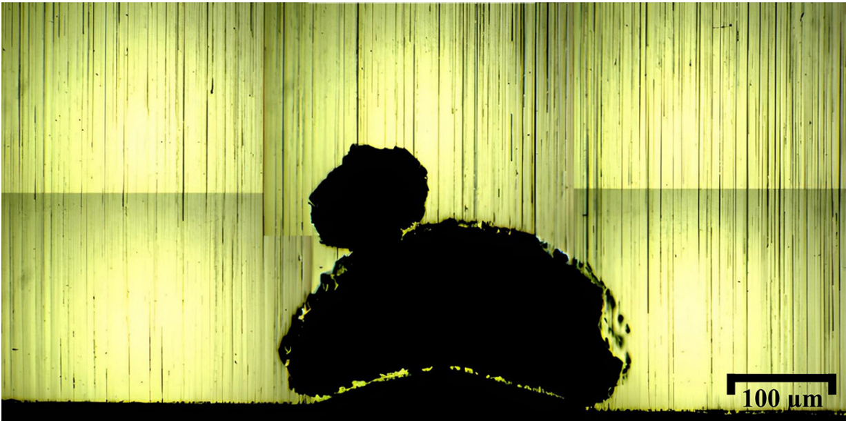
Figure 9. Cross-sectional morphology of secondary pit growth.
