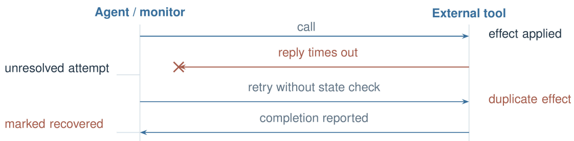
Figure 1. Analytical cross-layer failure chains: (A) stale state, (B) instruction-authority violation, and (C) unsafe recovery. These schematics show possible propagation paths and intervention points, not measured incidents.
