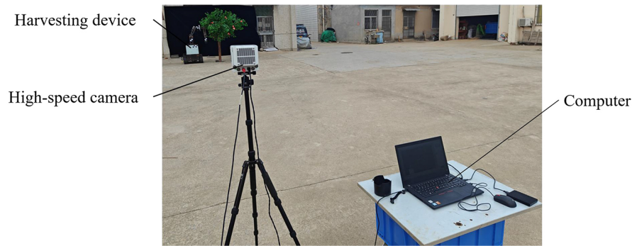
Figure 13. Experimental setup for boundary reference point tracking. Photograph taken by the authors.
