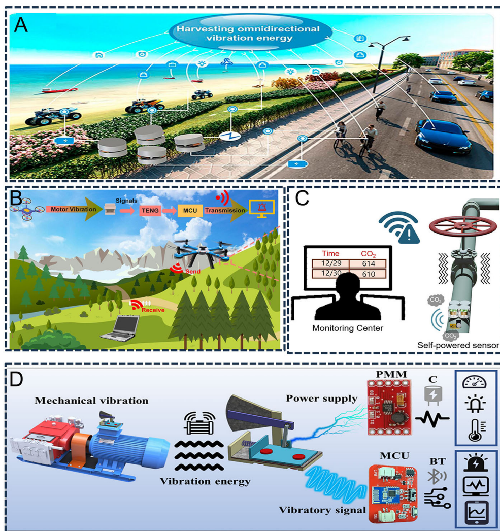
Figure 5. Application demonstrations of S-TENGs. (A) Omnidirectional hybrid energy harvesting for portable electronics. Used with permission [45] . Copyright 2022 American Chemical Society. (B) UAV vibration sensing and early warning generation. Used with permission [16] . Copyright 2024 Elsevier. (C) Pipeline-driven wireless carbon dioxide monitoring. Used with permission [25] . Copyright 2025 Elsevier. (D) Industrial equipment monitoring with predictive maintenance. Used with permission [44] . Copyright 2024 by the authors (CC BY 4.0).
