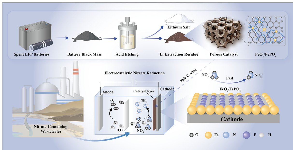
Figure 1. Schematic of the top-down reconstruction strategy for upcycling Spent \text{LiFePO}_4 (S-LFP) slags into electrocatalysts. Lithium extraction from S-LFP cathodes yields a solid slag that is conventionally discarded. Through acid-leaching-induced structural reconstruction, this low-value slag is transformed into a disordered Fe-P-O matrix (denoted HS-LFP) that serves as an efficient catalyst for electrocatalytic nitrate reduction to ammonia. The proposed local structural model of HS-LFP contains highly dispersed \text{Fe-O}_x species, neighboring Fe-O coordination motifs, and short-range ordered \text{FePO}_4 -related domains within a reconstructed Fe-P-O matrix. LFP: \text{LiFePO}_4 . HS-LFP: the S-LFP-derived slag.
