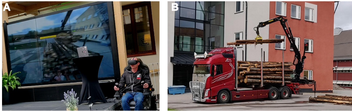
Figure 10. Photo of VR-goggle based crane operation from a remote location. (A) Operator with a VR headset and two joysticks. Operator's view is shown on the adjacent display; (B) The remotely operated crane [61] . VR: Virtual reality.
