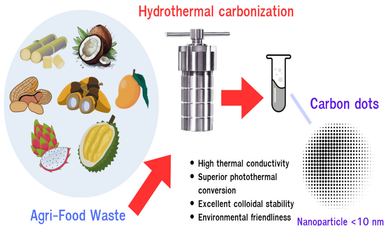
Figure 1. Concept to produce carbon dots by hydrothermal carbonization. The specific graphic icons used in Figure 1 (representing the agri-food waste raw material, the test tube, and the black carbon dots) were obtained from Canva ( https://www.canva.com ) under the platform's 'Free' user license.
