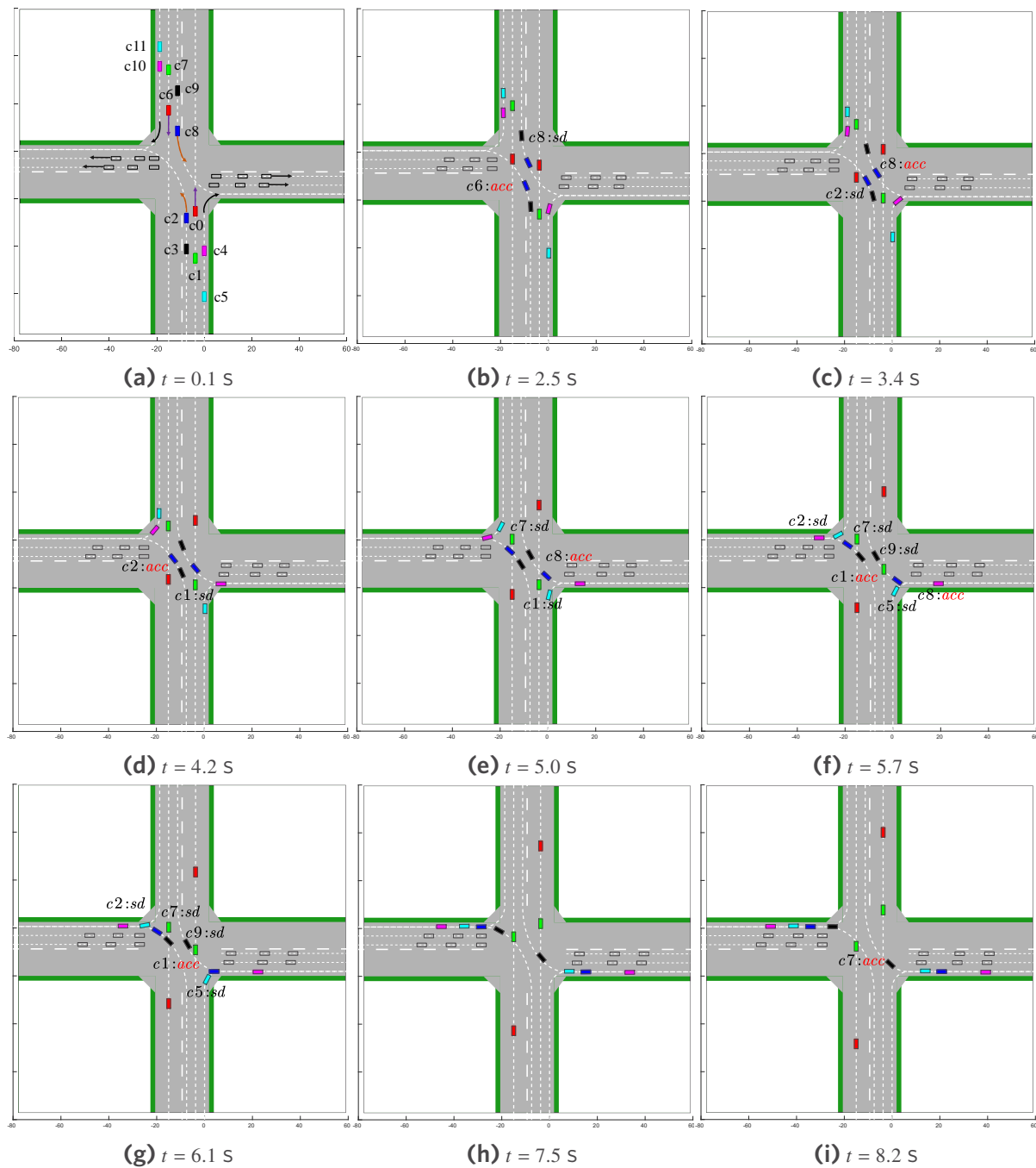
Figure 12. The cooperative decision-making and motion trajectories of MAVs at typical time instants in scenario 3. MAVs: Multiple autonomous vehicles.
