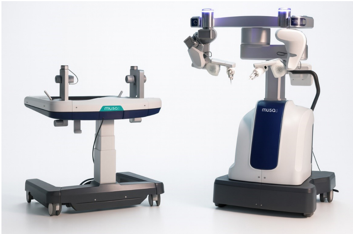
Figure 2. MUSA® 3 microsurgical robotic systems for robot-assisted micro- and supermicrosurgery (MicroSure B.V., Eindhoven, The Netherlands).
