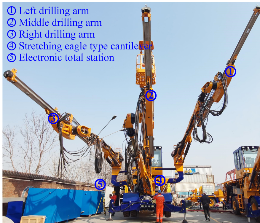
Figure 10. The structure of the experimental multi-arm drilling jumbo platform.
