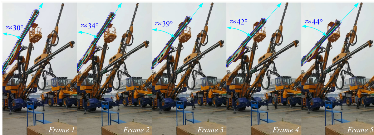
Figure 11. Continuous motion frames in planning experiment of the right drilling arm.
