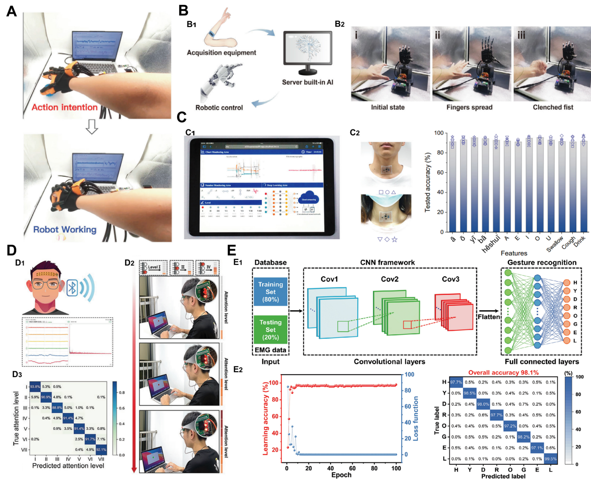
Figure 2. (A) Real-time active rehabilitation system based on dual-modality sensing of muscle force and sEMG [17] . Reprinted with permission. Copyright 2023, John Wiley & Sons; (B) Antibacterial hydrogel electrodes for prosthetic control in HMI applications: B 1 System operation schematic; B 2 Real-time prosthetic hand control via dual-channel sEMG signals [34] . Reprinted with permission. Copyright 2025, American Chemical Society; (C) Throat motion monitoring and rehabilitation using sEMG and accelerometer-based dual-modality sensing: C 1 Cloud-based interface for real-time throat motion tracking; C 2 Classification accuracy of 13 throat movements from two subjects [29] . Reprinted with permission. Copyright 2023, Springer Nature; (D) Continuous attention level assessment system: D 1 Schematic of wireless EEG acquisition system; D 2 Confusion matrix of attention classification results; D 3 Real-time system interface for sustained attention evaluation [19] . Reprinted with permission. Copyright 2023, John Wiley & Sons; (E) Machine learning-assisted sign language recognition based on sEMG: E 1 CNN-based algorithm framework for sign language translation; E 2 Post-training accuracy/loss curves and confusion matrix for eight sign gestures [24] . Reprinted with permission. Copyright 2024, John Wiley & Sons. HMI: Human-machine interaction; sEMG: surface electromyograms; EEG: electroencephalograms; CNN: convolutional neural network.
