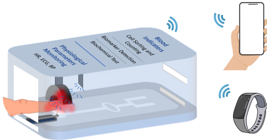
Figure 3. Simultaneous detection of biomarkers and physiological parameters from a finger.
