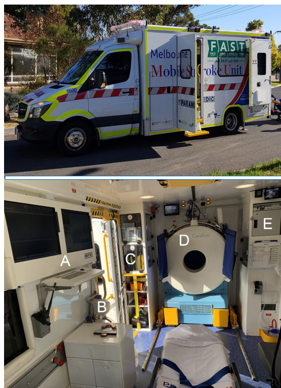
Figure 1. Melbourne mobile stroke unit exterior and interior. mobile stroke unit interior hardware: monitors for viewing and sending imaging in real-time (A); contrast injector (B); storage compartments for medications (C); CereTom scanner (D); contrast warmer (E).
