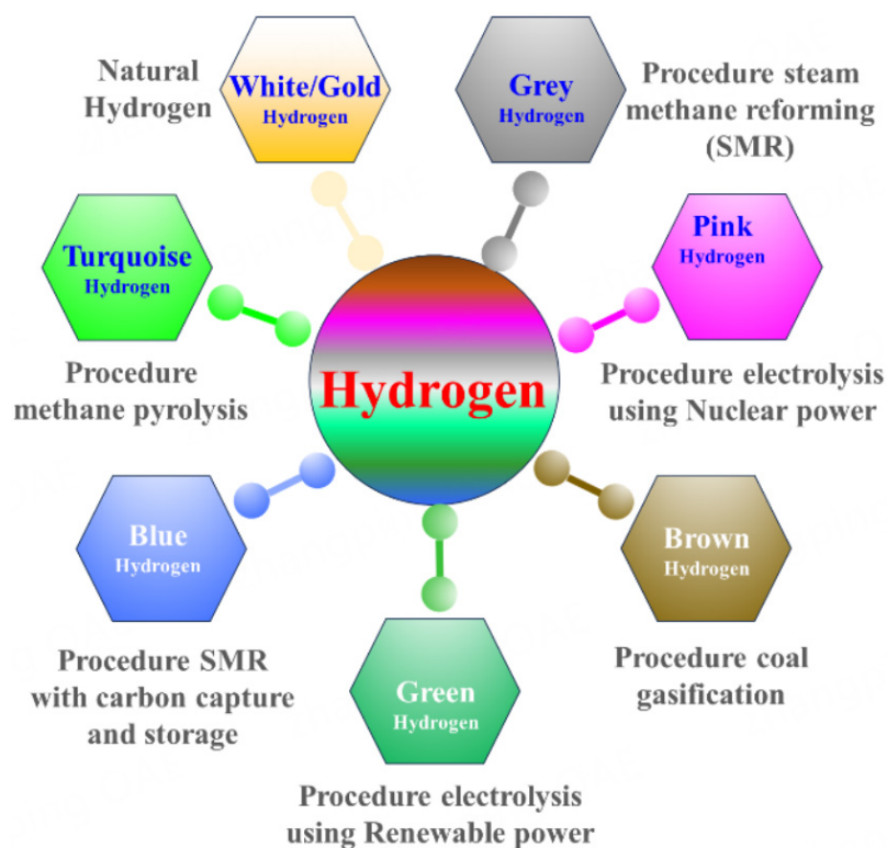
Figure 1. Classification of hydrogen production into seven types based on process and resource involvement.
