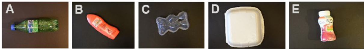
Figure 2. Examples of different types of plastics from the WaDaBa dataset in Figure 1. (A) Class 1 representing PETE (polyethylene terephthalate); (B) Class 2 representing HDPE (high-density polyethylene); (C) Class 5 representing PP (polypropylene); (D) Class 6 representing PS (polystyrene); (E) Class 7 representing Others [15] .
