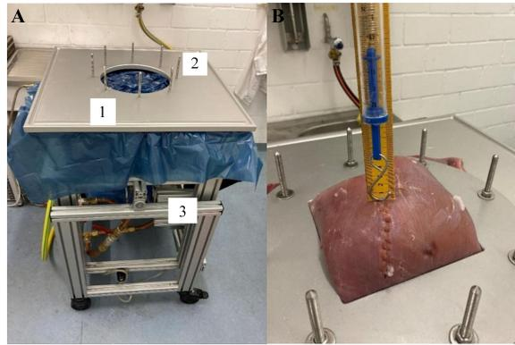
**Figure 1.** (A) Photo of the bench test and its elements (1: water cylinder with cover plate, 2: tank opening where pressure impacts are applied to the mounted tissue, 3: base frame with pipe system including inlet and outlet valves and pressure tank); (B) Mounted sutured tissue on the bench test during maximum pressure impact, suture tension is measured.
