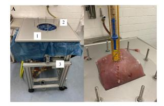
**Figure 1.** (A) Photo of the bench test and its elements (1: water cylinder with cover plate, 2: tank opening where pressure impacts are applied to the mounted tissue, 3: base frame with pipe system including inlet and outlet valves and pressure tank); (B) Mounted sutured tissue on the bench test during maximum pressure impact, suture tension is measured.
