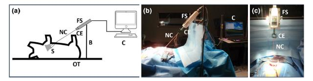
**Figure 3.** Illustration of the force measurement system developed: (a) schematic diagram of the test set-up; (b) lateral view of the test set-up during force quantification after mitral valved stent implantation; (c) frontal view of the FS connected to the NC via the CE. S: stent; NC: neo-chords; FS: force sensor; CE: connecting element; B: fixation bridge; C: computer for digital data recording<sup>[10]</sup>
