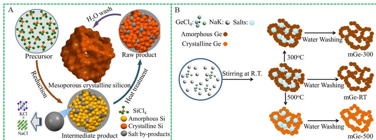
Figure 6. (A) Schematic of synthesis route of mesoporous crystalline Si. Reproduced with permission [67] (Copyright 2014, Nature Publishing Group). (B) Synthetic route of mesoporous Ge. Reproduced with permission [68] (Copyright 2020, Elsevier Inc.).
