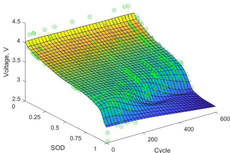
**Figure 2.** Comparison between SVM regression and datapoints. The surface represents the SVM regression. The datapoints used as Support Vectors are highlighted in green. SVM: support vector machine; SOD: state of discharge. The cycle is the number of times the battery has been charged and discharged throughout its lifetime.
