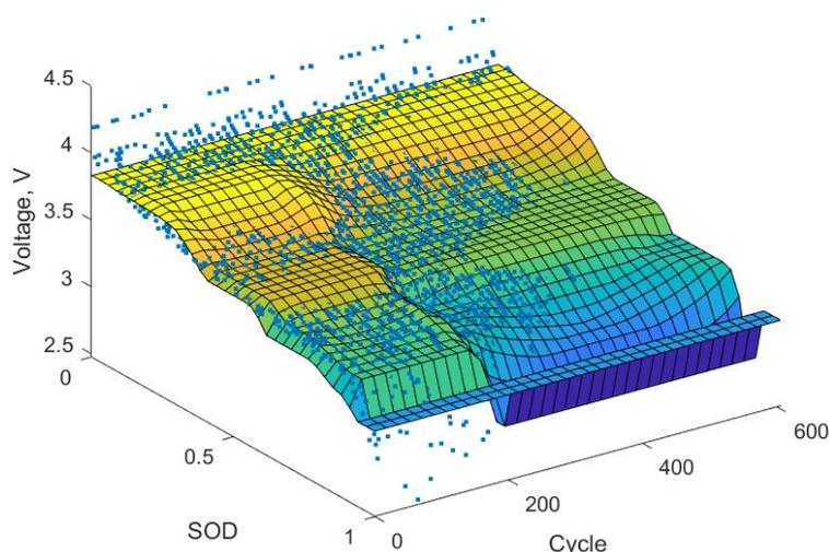
**Figure 4.** Comparison between FIS regression and datapoints. The surface represents the FIS regression. FIS: Fuzzy Inference System; SOD: state of discharge. The cycle is the number of times the battery has been charged and discharged throughout its lifetime.
