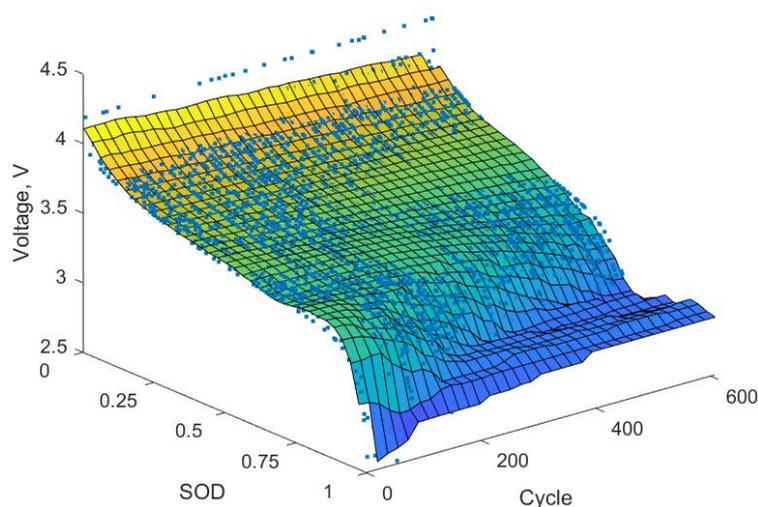
**Figure 3.** Comparison between RVM regression and datapoints. The surface represents the RVM regression. RVM: relevance vector machine; SOD: state of discharge. The cycle is the number of times the battery has been charged and discharged throughout its lifetime.
