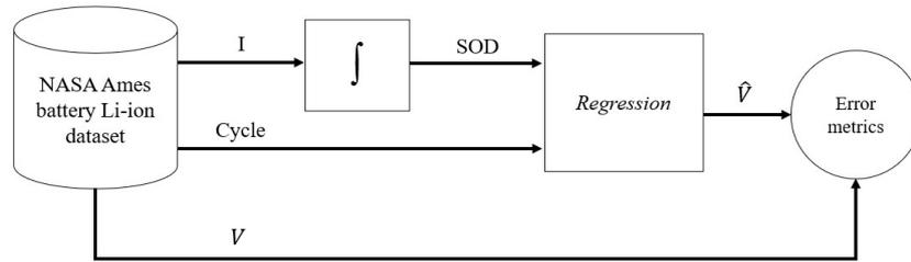
**Figure 1.** Data flowchart of the process.  $I$  stands for current and  $SOD$  stands for State of Discharge. The integral symbol represents the Coulomb counting method, which integrates current to obtain the SOD.  $v$  is the labeled voltage and  $\hat{v}$  is the estimated voltage.
