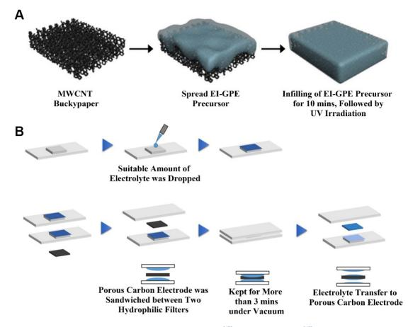
**Figure 4.** (A) Schematic illustrations for part of the preparation of EI-SC<sup>[47]</sup>. Reproduced from Ref.<sup>[47]</sup> with permission from Elsevier. (B) Schematic illustration of the stamping method<sup>[48]</sup>. Reproduced from Ref.<sup>[48]</sup> with permission from American Chemical Society. MWCNT: Multi-walled carbon nanotubes; EI-GPE: organic gel polymer electrolyte; EI-SC: flexible supercapacitor.
