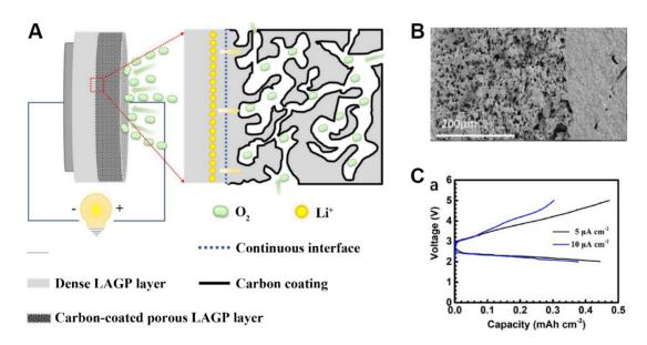
**Figure 9.** (A) Schematic diagram of LOB with integrated structure. (B) Cross section of structure. (C) Galvanostatic discharge and charge curves of the novel LOB, with currents of 5 and 10  $\mu$ A cm<sup>-2</sup> between 2 and 5 V<sup>[56]</sup>. Reproduced from Ref.<sup>[56]</sup> with permission from IOP Publishing. LAGP: Li<sub>15</sub>Al<sub>05</sub>Ge<sub>15</sub>P<sub>3</sub>O<sub>12</sub>.
