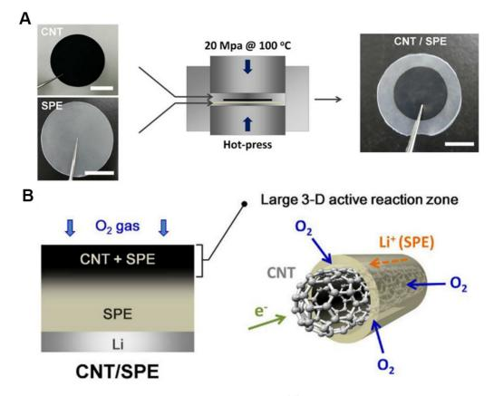
**Figure 6.** (A) Optical images and schematic of preparation of 3D CNT/SPE<sup>[53]</sup>. (B) Enlarged 3D active reaction zone in 3D CNT/SPE architecture<sup>[53]</sup>. Reproduced from Ref.<sup>[53]</sup> with permission from Springer Nature. CNT: Carbon nanotube; SPE: solid polymer eletrolyte.
