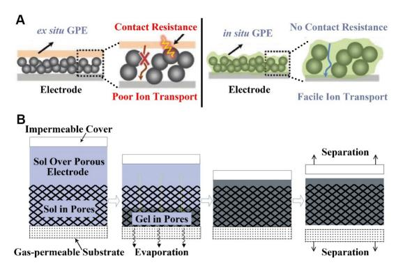
**Figure 3.** (A) *Ex situ* GPE *vs.in situ* GPE, with *in situ* GPE having higher ionic conductivity<sup>[44]</sup>. Reproduced from Ref.<sup>[44]</sup> with permission from John Wiley and Sons. (B) Schematic diagram of bottom-up infilling method<sup>[45]</sup>. Reproduced from Ref.<sup>[45]</sup> with permission from Springer Nature. GPE: Gel polymer electrolyte.
