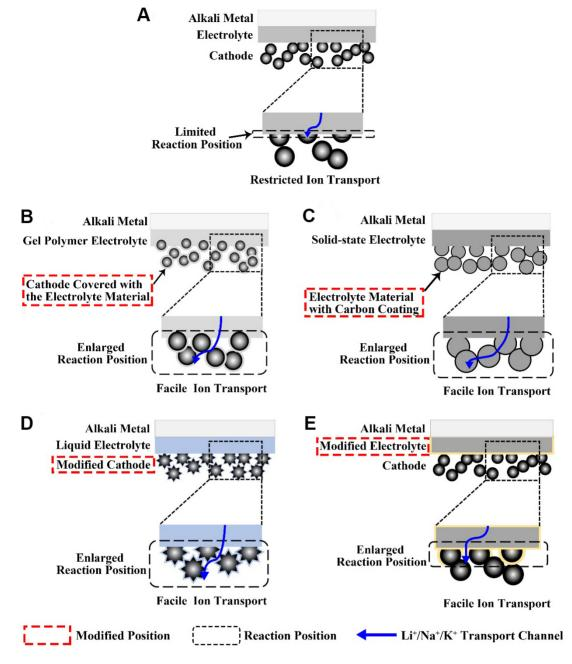
**Figure 1.** (A) Battery with sandwich structure. Schematic overview of four different approaches to engineer the electrolyte layercathode interface: (B) mixing electrolyte and cathode grains; (C) integration of electrolyte and cathode materials; (D) modification of cathode structure; and (E) modification of electrolyte.
