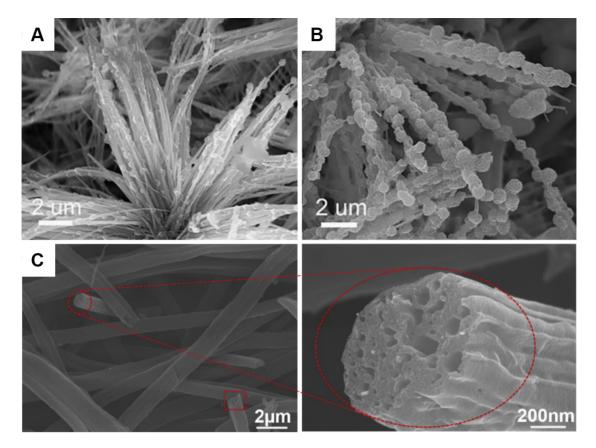
**Figure 11.** SEM images of (A) half and (B) fully discharged  $Co_9S_8$  nanorods<sup>[36]</sup>. Reproduced from Ref.<sup>[36]</sup> with permission from John Wiley and Sons. (C) SEM images of the cathode obtained by electrospinning at magnifications of 2  $\mu$ m and 200 nm<sup>[64]</sup>. Reproduced from Ref.<sup>[64]</sup> with permission from Elsevier. SEM: Scanning electron microscopy.
