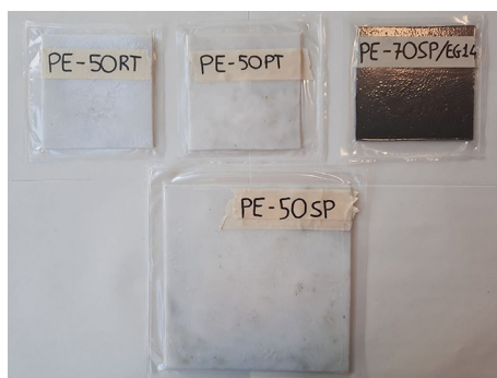
Figure 8. PE enveloped panels having dimensions 120 \times 120 \times 3 \text{ mm}^3 (top) and 200 \times 200 \times 3 \text{ mm}^3 (bottom).
