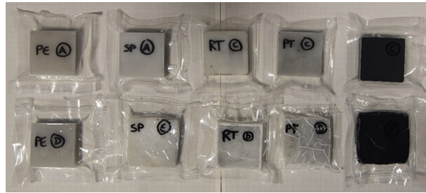
Figure 12. Compression tested samples at 30 °C (above) and 80 °C (below). From left to right: neat HDPE, PE-50SP, PE-50RT, PE-50PT and PE-70SA/EG14.
