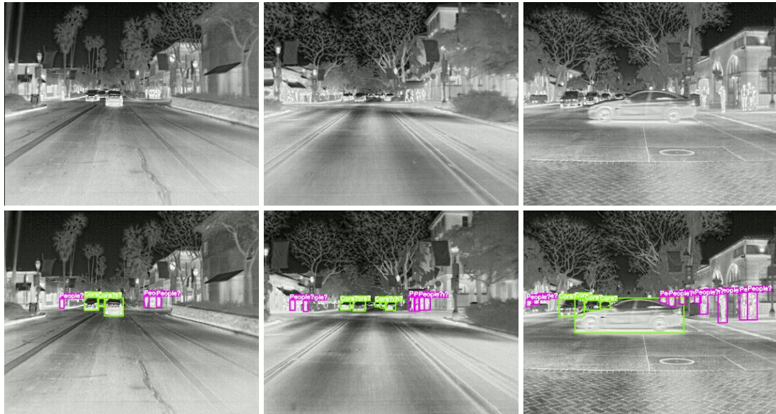
Figure 8. Some examples of the detection result on the FLIR dataset. The first column is the original image, and the second column is the result of MobileNetV3-YOLOv4.
