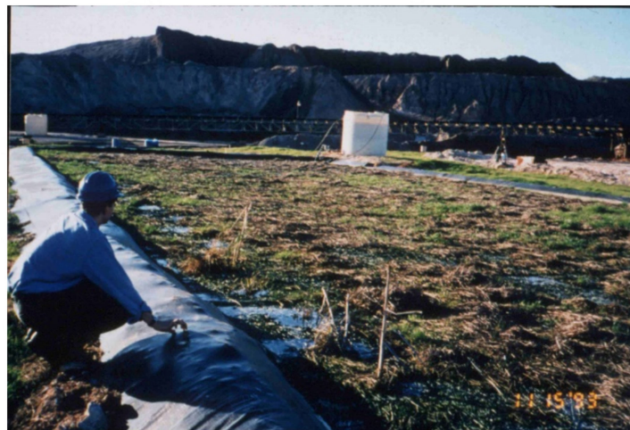
Figure 4. Hay seed germination on BCR surface. BCR: Biochemical reactor.
