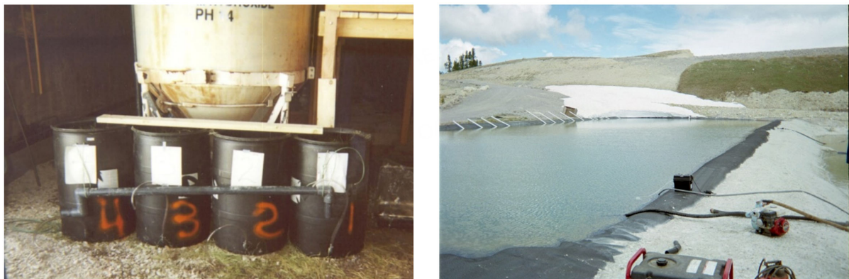
Figure 10. Luttrell bench BCRs and demonstration BCR in spring. BCR: Biochemical reactor.
