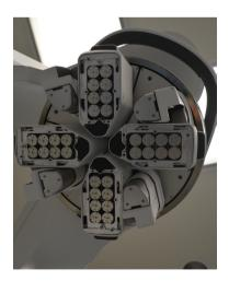
Figure 6. Single port instrument insertion platform
