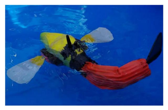
Figure 7. A rigid-soft coupled robot fish in BCF-MPF propulsion mode<sup>[31]</sup>. BCF: Body and/or caudal fin; MPF: median and/or paired fin.
