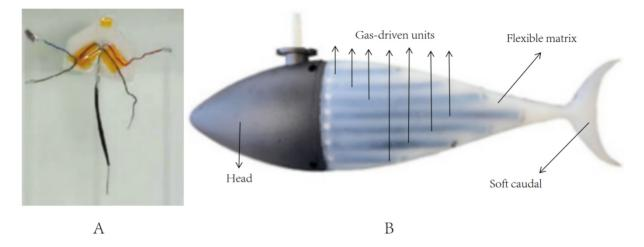
**Figure 3.** Soft robot fishes in BCF propulsion mode: (A) a robot fish with DEAs<sup>[20]</sup>; and (B) Flexi-Tuna<sup>[21]</sup>. BCF: Body and/or caudal fin; DEAs: dielectric elastomer actuators.
