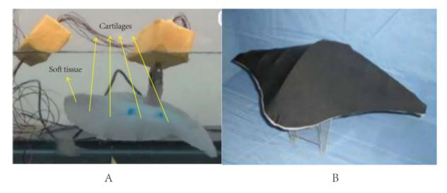
**Figure 5.** Rigid-soft coupled robot fishes in MPF propulsion mode: (A) a robot fish with soft tissue and cartilages.<sup>[27]</sup>; and (B) bionic cownose ray robot fish<sup>[28]</sup>. MPF: Median and/or paired fin.
