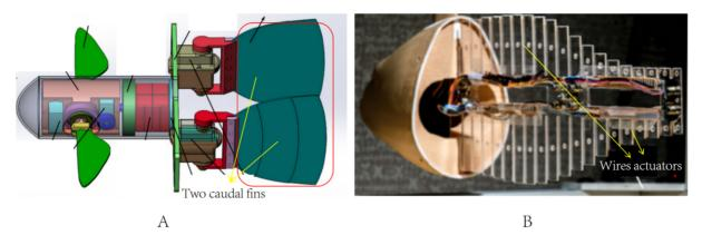
**Figure 4.** Rigid-soft coupled robot fishes in BCF propulsion mode: (A) a robot fish with two caudal fins<sup>[22]</sup>; and (B) wires actuators of the robot fish<sup>[23]</sup>. BCF: Body and/or caudal fin.
