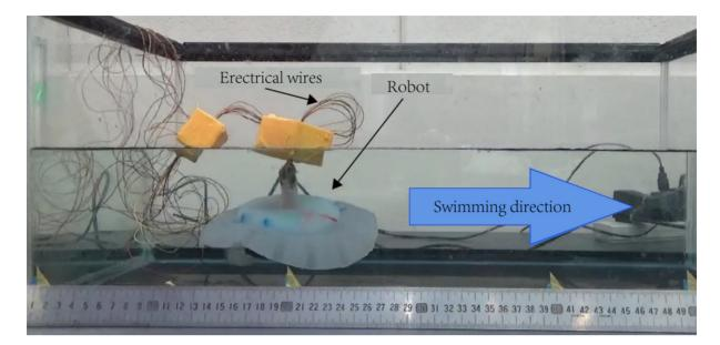
Figure 8. Experimental setup for measuring the swimming speed<sup>[27]</sup>.
