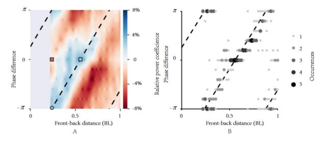
**Figure 11.** The following robot fish saves energy by vortex phase matching. (A) Relative power coefficient: Positive and negative values, respectively, represent energy saving and energy cost relative to swimming alone. The dashed line represents the function between phase difference and front-back distance, as shown in (B). (B) Location of energy saving: The size and darkness of the dots represent the number of times that the energy saving state occurs<sup>[50]</sup>.
