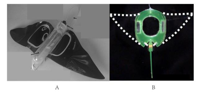
**Figure 6.** Soft robot fishes in BCF-MPF propulsion mode: (A) a soft robot fish<sup>[29]</sup>; and (B) a soft electronic fish<sup>[30]</sup>. BCF: Body and/or caudal fin; MPF: median and/or paired fin.
