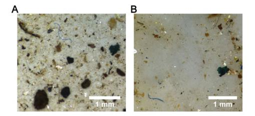
Figure 4. Sediment sample (A) before and (B) after biogenic organic matter removal using 10 mL of 30% hydrogen peroxide and 10 mL of 0.05 M of iron catalyst for 15 min.
