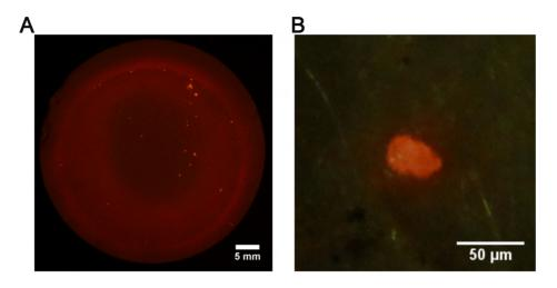
**Figure 5.** Fluorescent microplastics after Nile Red staining and under 470 nm with an orange lens filter: full glass fiber filter (47 mm) spiked with (A) microplastics and (B) suspected microplastics in river water under the microscope.
