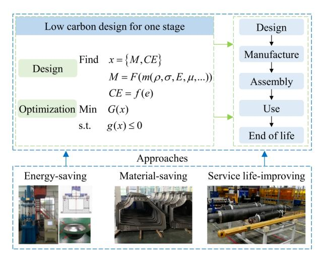
**Figure 3.** The framework of low carbon design. (*x* is a variable related to mass (*M*) and energy consumption (*CE*); every mass *M* has its corresponding attributes, which are density  $\rho$ , material strength  $\sigma$ , the elastic modulus *E*, and Poisson's ratio  $\mu$ , etc.; *CE* is related to energy consumption factor *e*; *G*(*x*) is the carbon emission and the objective function; *g*(*x*) is the constraint function).
