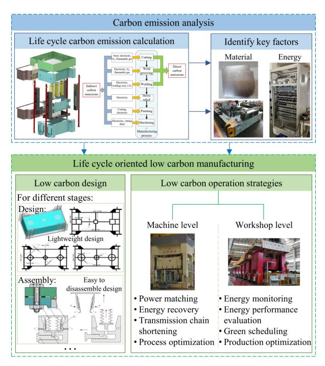
Figure 1. Framework of the life cycle-oriented low carbon manufacturing of mechanical equipment.
