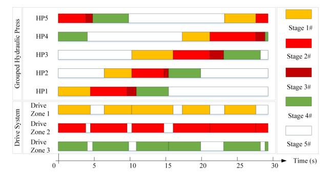
**Figure 16.** Working status of the drive system for grouped hydraulic press<sup>[56]</sup>. (in the figure, Stage 1#: FF; Stage 2#: P; Stage 3#: PM; Stage 4#: R; and Stage 5#: I).
