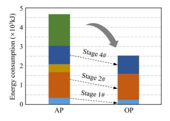
Figure 17. Energy consumption for a single press (AP) and one hydraulic press (OP) in the group<sup>[57]</sup>.
