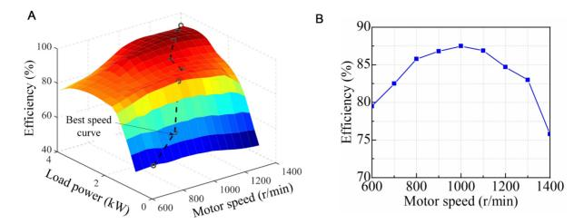
Figure 14. Energy efficiency of drive unit changing with motor speed under (A) variable load power, and (B) given load power at 2  $kW^{[54]}$ .
