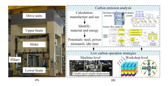
Figure 6. (A) A 2000-ton rapid sheet tension hydraulic press and (B) life cycle oriented low carbon manufacturing technology route of the hydraulic press.
