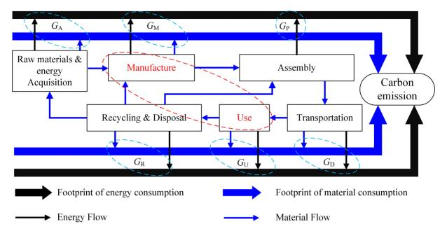
Figure 2. The carbon footprint of mechanical equipment in its life cycle.
