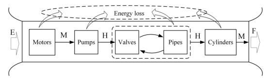
**Figure 9.** The basic energy flow of the hydraulic press system in use<sup>[53]</sup> (E is for electrical energy, M is for mechanical energy, H is for hydraulic energy, and F is for forming energy).
