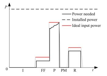
**Figure 11.** Demanded power of all stages in a forming process<sup>[29]</sup>. I: Idle; FF: fast falling; P: press; PM: pressure maintaining; and R: returning.
