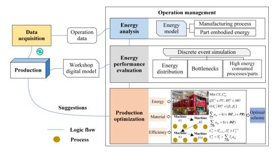
Figure 5. An integrated framework to support low carbon manufacturing on the workshop level.
