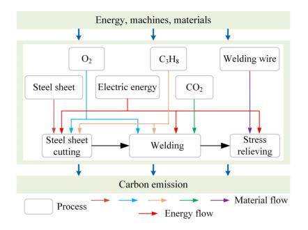
Figure 7. System boundary of carbon emissions in the manufacturing process of the hydraulic press<sup>[52]</sup>.
