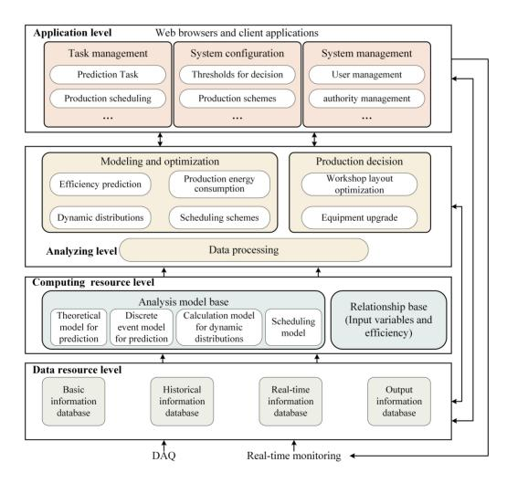
Figure 20. Functional architecture of the software.
