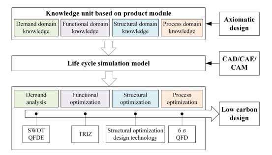
Figure 19. Tools and method integration in life cycle oriented low carbon manufacturing.
