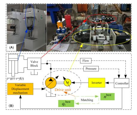
**Figure 13.** (A) Experimental platform and (B) control schematic diagram for the drive unit of variable displacement and variable speed<sup>[54]</sup> ( $q_t^{best}$  is the displacement of the pump and  $n^{best}$  is the speed of the motor in combination with maximum energy efficiency).
