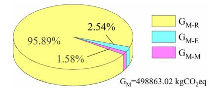
**Figure 8.** Distribution of carbon emissions in the manufacturing stage of the hydraulic press. ( $G_M$  is the carbon emissions of raw materials,  $G_{M-E}$  is the carbon emissions derived from energy consumption during manufacturing processes, and  $G_{M-M}$  is the direct carbon emissions in the processes).
