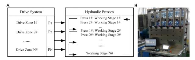
**Figure 15.** (A) Physical architecture of the energy matching method<sup>[55]</sup> and (B) pneumatic experimental prototype. (In the figure, the drive system is divided into *N* drive zones according to the number of working stages of the hydraulic press in a forming process; and the output power *Pi* of each drive zone matches the required power of the hydraulic press working in the corresponding working stage).
