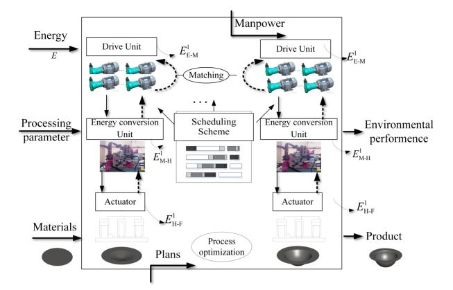
Figure 12. Low carbon operation strategies in a hydraulic press production line.
