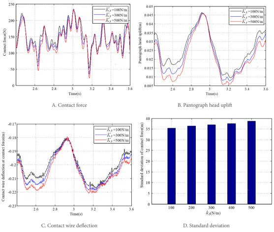
**Figure 26.** Results of the pantograph-overhead system dynamic response with different  $K_3$ .
