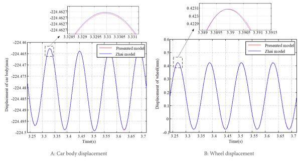
Figure 3. Verification of the vehicle-track model.
