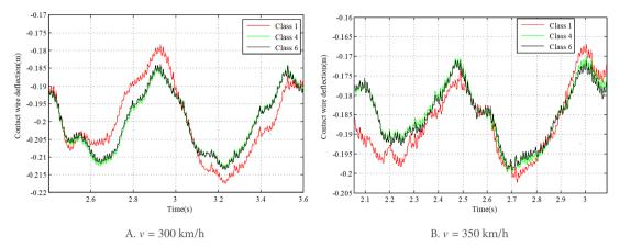
Figure 18. Results of contact wire deflection at contact point with different types of track irregularities.
