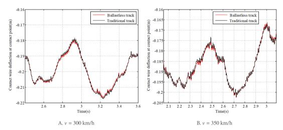
Figure 23. Comparison of contact wire deflection at contact point between traditional tack and ballastless track.
