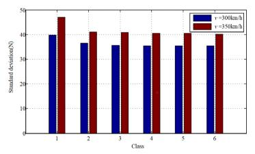
Figure 19. The results of standard deviation of contact force with different qualities of track irregularities.
