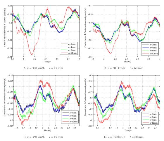
Figure 8. Results of contact wire deflection at contact point at different wave depths of rail irregularity.
