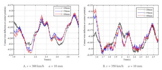
Figure 12. Results of contact wire deflection at contact point at different wavelengths of rail irregularity.
