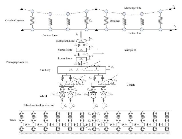
Figure 1. Vertical coupling model for overhead system-pantograph-vehicle-track system.
