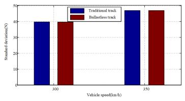
Figure 24. Results of standard deviation of contact force with traditional tack and ballastless track.
