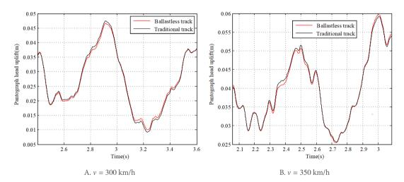
Figure 22. Comparison of pantograph head uplift between traditional tack and ballastless track.
