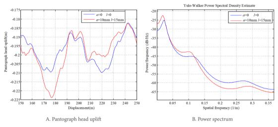
Figure 15. Pantograph head uplift and its spectral estimation.
