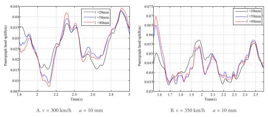
Figure 11. Results of pantograph head uplift at different wavelengths of rail irregularity.
