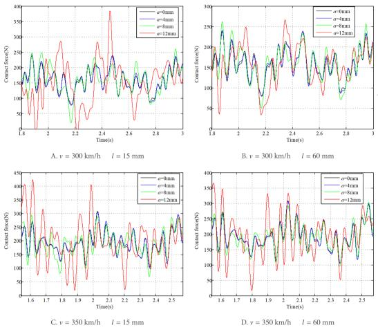
Figure 6. Results of contact force at different wave depths of rail irregularity.
