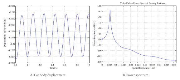
Figure 14. Car body displacement and its power spectrum.
