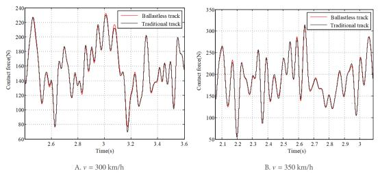
Figure 21. Comparison of contact force between traditional tack and ballastless track.
