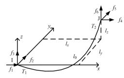
Figure 2. Nonlinear cable element.
