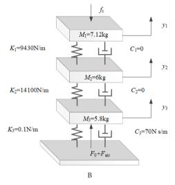
Figure 4. Parameters of the pantograph-overhead system: (A) geometry information of a simple overhead system model; and (B) three-DOF model of a pantograph.
