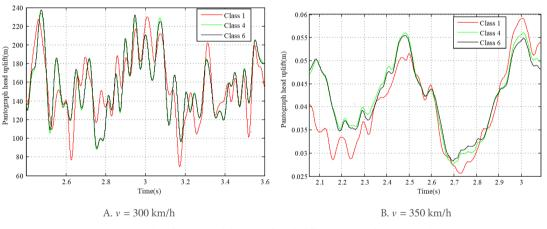
Figure 17. Results of pantograph head uplift with different types of track irregularities.
