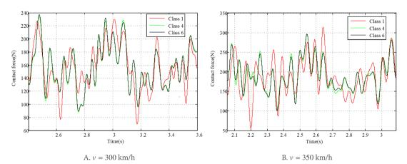
Figure 16. Results of contact force with different types of track irregularities.
