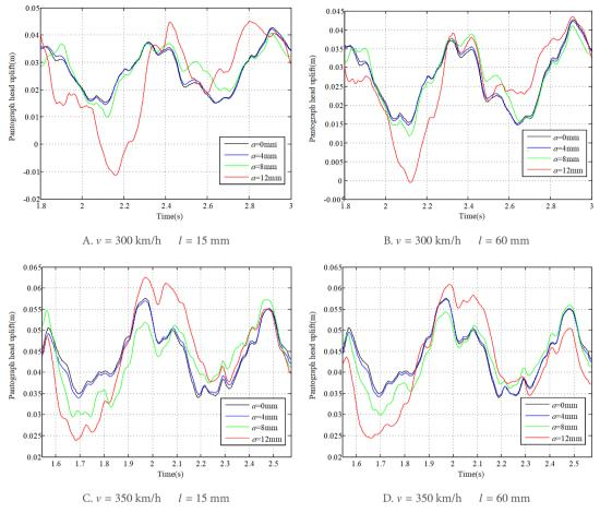
Figure 7. Results of pantograph head uplift at different wave depths of rail irregularity.
