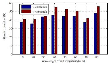
Figure 13. Results of standard deviation of contact force at different wavelengths of rail irregularity.
