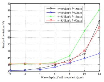
Figure 9. Standard deviation and statistical minimum value of contact force at different wave depths of rail irregularity.
