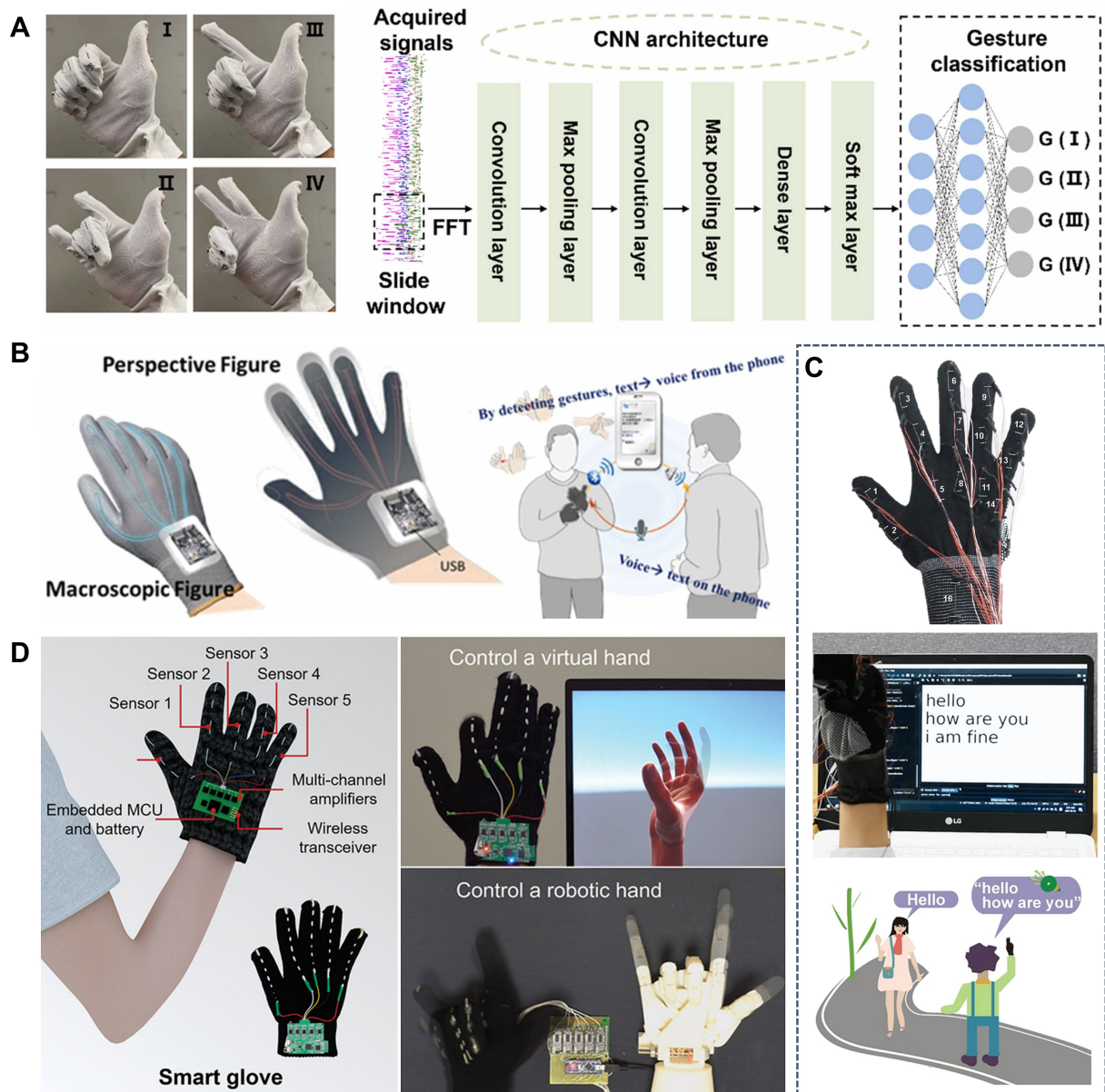
Figure 11. Application of multimodal electronic textiles in gesture interaction interface. (A) A smart glove with a fiber sensor for hand gesture identification by deep learning networks. Reproduced with permission [193] . Copyright 2022, Elsevier; (B) schematic diagram of smart glove framework and working mode for gesture interaction. Reproduced with permission [194] . Copyright 2022, Elsevier; (C) sign-language translation glove for a signer communicating with a person. Reproduced with permission [195] . Copyright 2022, The Author(s), published by Springer Nature; (D) a smart data glove for human-machine gesture collaboration, including control of a virtual hand and control of a robotic hand. Reproduced with permission [196] . Copyright 2021, Wiley-VCH.
