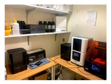
Figure 1. 3D printer lab. An example of a clinic-based 3D printing lab demonstrating several different printers and post-print-processing equipment.
