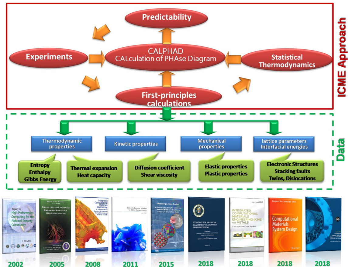
Figure 3. Proposed data-driven ICME approach together with the corresponding foundations and milestones [29] . ICME: Integrated Computational Materials Engineering.
