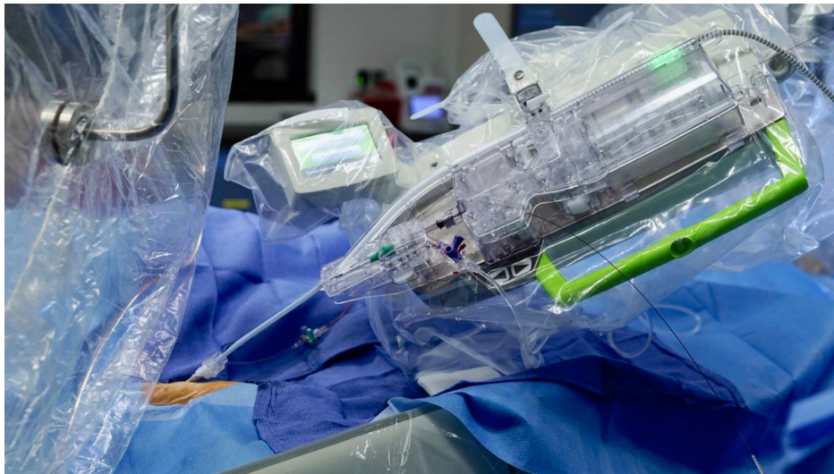
Figure 1. CorPath GRX system assisting in coronary intervention, reprinted with permission of Siemens Healthineers [6] (published with permission of Siemens Healthineers).
