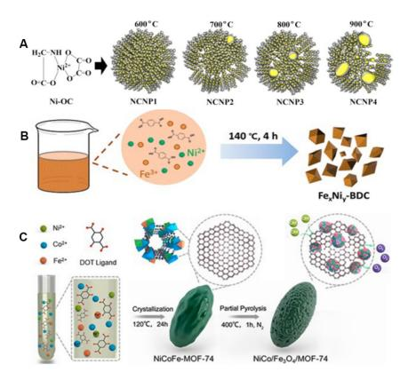
**Figure 8.** (A) Schematic representation of NCNP composite synthesis. (B) Schematic of FexNiy-BDC synthesis. (C) Schematic of NiCo/Fe<sub>3</sub>O<sub>4</sub>/MOF-74 synthesis. Reproduced with permission. Copyright 2019, Elsevier<sup>[102]</sup>.
