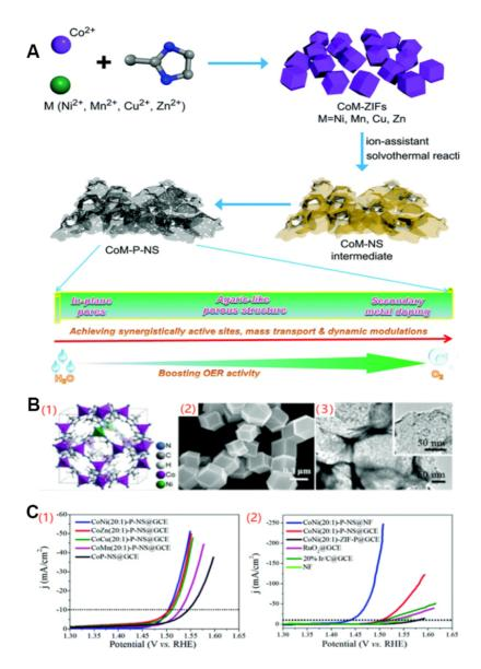
**Figure 6.** (A) Schematic illustration of a general synthetic approach to CoM-P NSs for high-efficiency OER derived from bimetallic MOFNs. (B) (1) Crystal structure, (2) SEM image of CoNi(20:1)-ZIF precursor and (3) TEM. (C) (1) Polarization curves of CoP-NS and CoM(20:(1)-P-NS (M = Ni, Mn, Cu or Zn) and of (2) CoNi(20:1)-P-NS on GCE or Ni foam (NF), CoNi(20:1)-ZIF-P. Reproduced with permission. Copyright 2017, Royal Society of Chemistry<sup>[91]</sup>.
