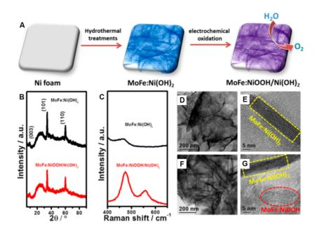
**Figure 2.** (A) Synthetic steps of forming MoFe:Ni(OH)<sub>2</sub>/NiOOH NSs on nickel foam directly. (B) XRD patterns of MoFe:Ni-(OH)<sub>2</sub> and MoFe:Ni(OH)<sub>2</sub>/NiOOH NSs. (C) Raman spectra of MoFe:Ni(OH)<sub>2</sub> and MoFe:Ni(OH)<sub>2</sub>/NiOOH NSs. (D-G) TEM and HRTEM images of MoFe:Ni(OH)<sub>2</sub> and MoFe:Ni-(OH)<sub>2</sub>/NiOOH NSs. Reproduced with permission. Copyright 2018, American Chemical Society<sup>[56]</sup>.
