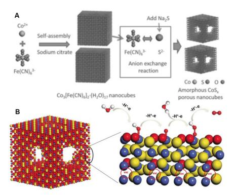
**Figure 7.** (A) Schematic of the synthesis process of  $A-CoS_{4,6}O_{0,6}$  PNCs. (B) Schematic of oxygen-containing amorphous cobalt sulfide porous nanocubes with Co-S dangling bands, a distorted  $CoS_{4,6}O_{0,6}$  octahedral structure and incorporated oxygen in the  $CoS_x$  (vac = vacancy, Co = blue, S = yellow, O = red and H = white). Reproduced with permission. Copyright 2017, Wiley<sup>[95]</sup>.
