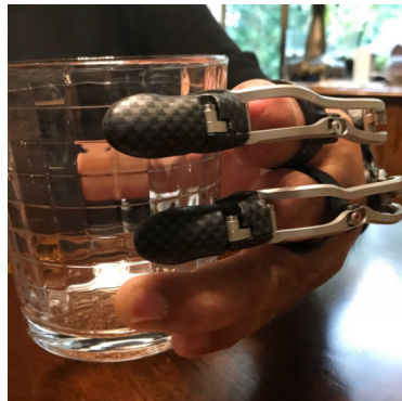
Figure 2. Naked Prosthetic MP Driver. Prosthesis is powered by residual motion at remnant MP joints.
