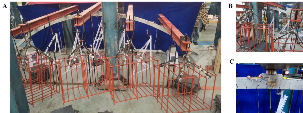
Figure 11. Experimental model. (A) Unloaded model; (B) 1/3L, 1/2L loading damage; (C) Accelerometers and arch loading point.
