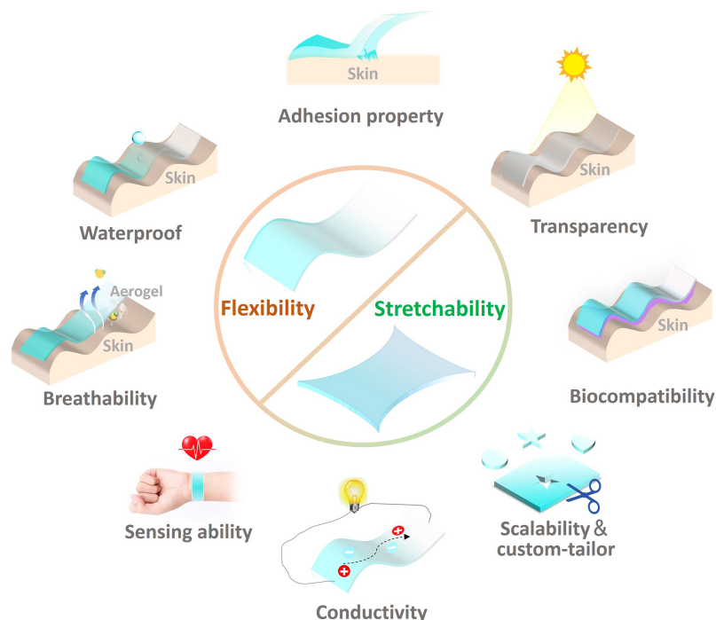
Figure 2. Schematic illustrating the unique characteristics of gel-based materials and devices reported in the literature.
