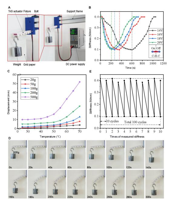
**Figure 4.** Characterization of tunable stiffness and load capacity of Tri-S actuator. (A) Experimental platform of stiffness test of Tri-S actuator. (B) Stiffness of Tri-S actuator as a function of electrified time. (C) Load capacity characterization of Tri-S actuator with temperature variations. (D) Dynamic variation process of load capacity of Tri-S actuator. (E) Measured stiffness range of actuator after multi-cycle actuation.
