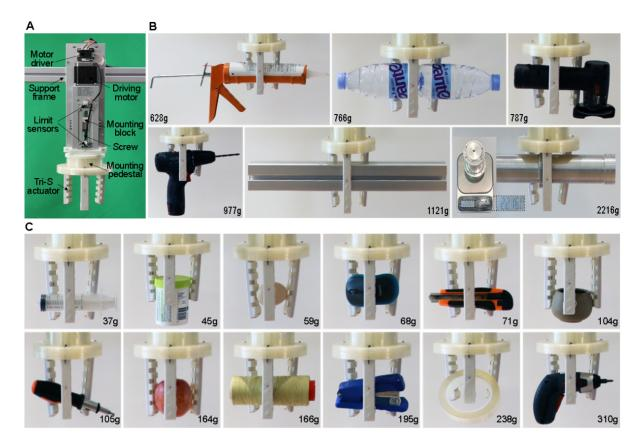
Figure 5. Exhibition of tunable-stiffness and shape-locking capacity of soft gripper. (A) Soft gripper equipped with Tri-S actuators. (B) Loading capacity test of soft gripper. (C) Shape locking capacity test of soft gripper.
