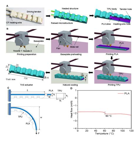
**Figure 1.** Design and fabrication of a Tri-S actuator. (A) Illustration of Tri-S actuator composition. (B) Tri-S actuator manufacturing processes by 3D-printed hybrid multi-material technology. (C) Description of Tri-S actuator with rectangular cross sections. (D) Test of Tg for PLA by differential scanning calorimetry analysis. PLA: polylactic acid; TPU: thermoplastic polyurethane.
