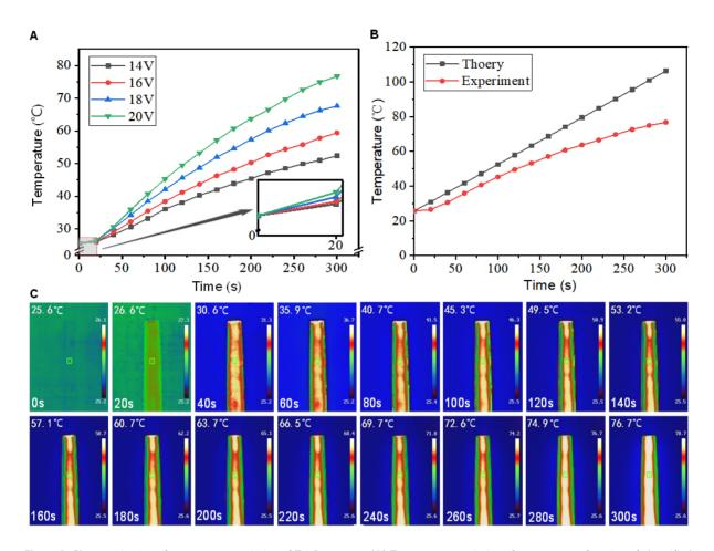
**Figure 2.** Characterization of temperature variation of Tri-S actuator. (A) Temperature variation of actuator as a function of electrified time. (B) Temperature comparison between theory and experiment. (C) Dynamic thermal states of Tri-S actuator at applied voltage of 20 V.
