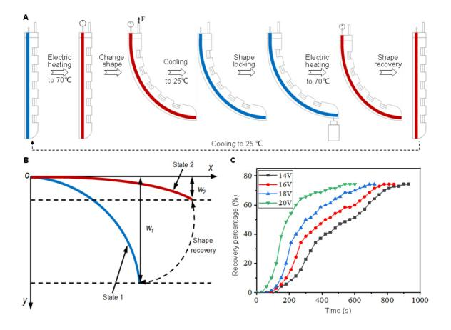
Figure 3. Shape recovery mechanism of Tri-S actuator. (A) Shape recovery process of actuator. (B) Schematic explanation of recovery rate. (C) Characterization of shape recovery under different applied voltages as a function of electrified time.
