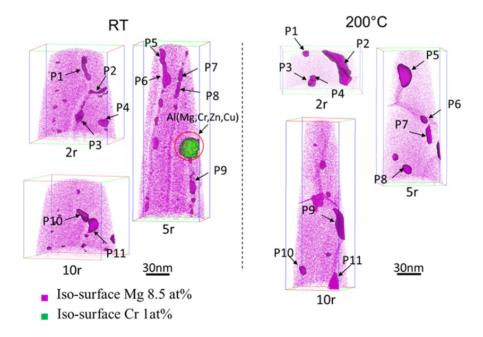
**Figure 4.** Three-dimensional reconstructed Mg atom maps of AA7075 samples processed by HPT in different conditions, with precipitates defined by iso-concentration surfaces at 8.5 at.% Mg (in pink) and 1.0 at.% Cr (in green). Reproduced with permission, Copyright 2018, Elsevier<sup>[20]</sup>.
