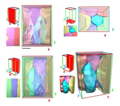
**Figure 3.** Tomographic view of nanostructural architecture in HPT 7075 alloy. Lineal and node solute structures are observed to occur at grain boundary interfaces and junctions. Reproduced with permission, Copyright 2010, Nature Publishing Group<sup>[12]</sup>.
