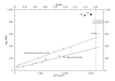
**Figure 2.** Hall-Petch relationships for Al 1100 and Al-3%Mg supported by the yield stress of nanostructured alloys Al-3%Mg, 1570 and 7475. Reproduced with permission, Copyright 2010, Elsevier<sup>[11]</sup>.
