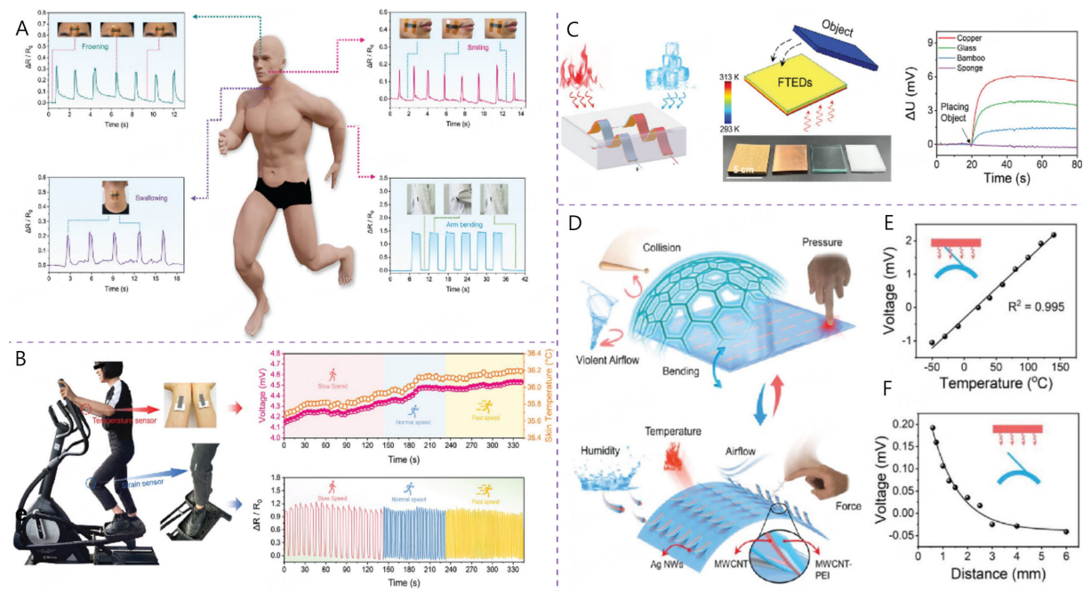
Figure 13. (A) Real-time monitoring of human motion with relative resistance variation of CAST-PTFE film at different human motions, and (B) real-time temperature and knee bending monitoring during human motion monitoring output voltage and relative resistance of CAST-PTFE film [232], Copyright 2024 Wiley-VCH GmbH (C) sensing object temperature and thermal conductivity of FTEDs and \Delta U -time curve for different objects [235], Copyright 2024 Wiley-VCH GmbH (D) various sensing modalities for 2D and 3D structures, and (E, F) voltage-temperature curves for the sensor in 3D mode and heat proximity test at 40 °C [236]. Copyright 2024 Wiley-VCH GmbH. FTEDs: Flexible thermoelectric device; PTFE: polytetrafluoroethylene.
