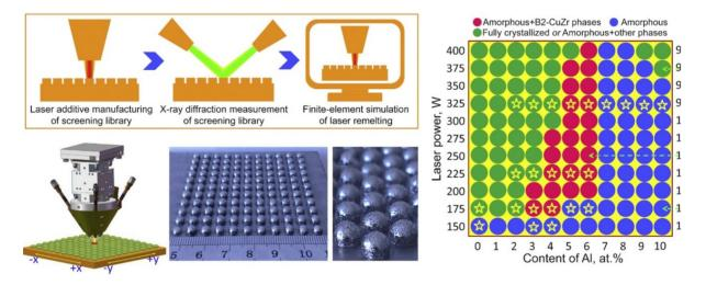
**Figure 3.** HT processing experiments using powder-based DED by Yu *et al.* Reproduced with permission. Copyright © 2021, Elsevier<sup>[12]</sup>. Samples are printed as a matrix with the change of Al content and laser power. Phase identifications were performed using the XRD technique. DED: Directed energy deposition; XRD: X-ray diffraction.
