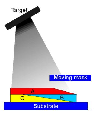
**Figure 2.** Illustration of the deposition procedure with a moving mask. A, B, and C are thin layer deposited on the substrate. Moving mask and rotation of substrate will help on the concentration control of metals deposited on the substrate. Figure is reproduced according to the work by Hui *et al.*<sup>(11)</sup>. Reproduced with permission. Copyright © 2019, The Author(s).
