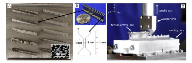
**Figure 5.** HT mechanical tests on tensile arrays printed using LPBF. Reproduced with permission. © 2019 Elsevier B.V. All rights reserved.<sup>(20)</sup>. (A) Printed tensile arrays of SS316L. (B) Tensile array after cutting from the substrate. (C) Dimension of the tensile bar for testing. (D) Set-up for HT tensile tests. LPBF: Laser powder bed fusion; HT: high-throughput.
