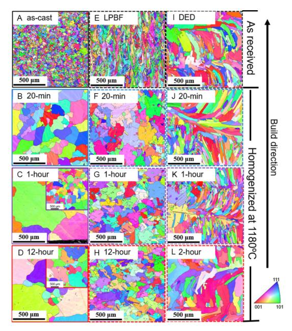
**Figure 6.** Comparison of grain structure in the Inconel 718 among different processing methods, suction cast (A-D), LPBF (E-H), and powder-based DED (I-L) based on IPF (inverse pole figure) maps of EBSD analysis. LPBF: Laser powder bed fusion; DED: directed energy deposition.
