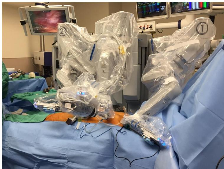
**Figure 3.** Robotic coronary artery bypass: docking of the Da Vinci robot.
