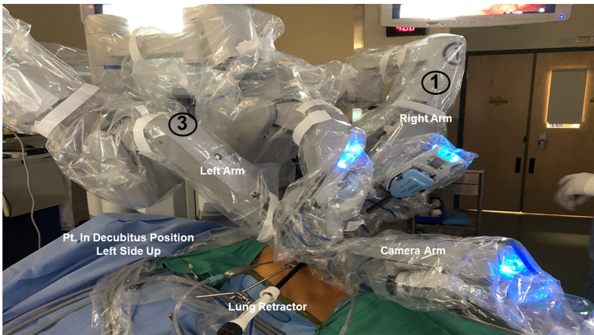
Figure 12. Left robotic selective sympathectomy. Intraoperative photograph depicts the robot in position. Three robotic arms are used
