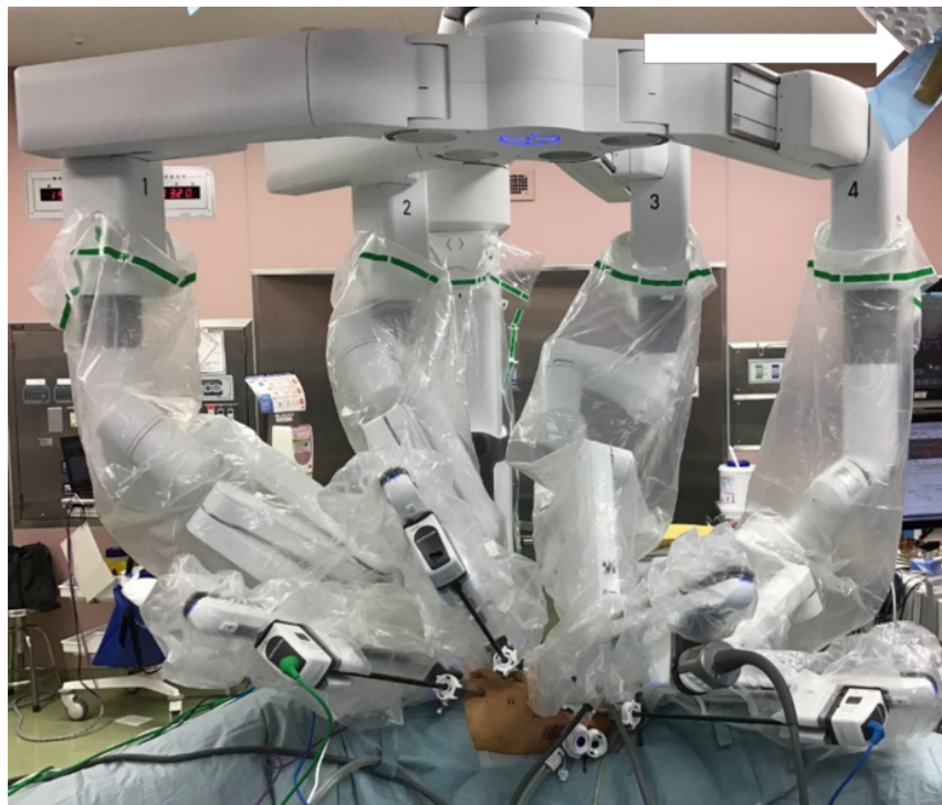
Figure 2. Final appearance after robot setup in robot-assisted thoracoscopic esophagectomy in lateral decubitus position. The patient cart is rolled in from the patient's dorsal side and docked to the robotic ports. Arrows indicate the cranial direction.
