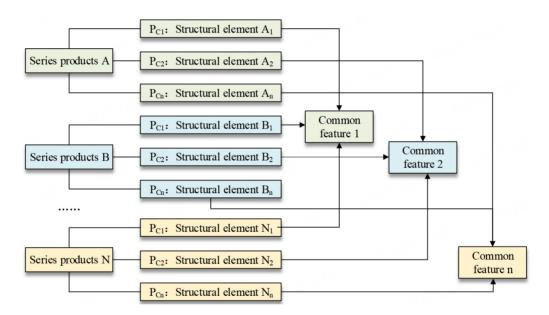
$\textbf{Figure 2.} \ \textbf{Schematic diagram of product structure feature extraction}.$
