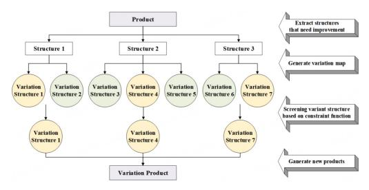
Figure 3. Schematic diagram of structural variation map generation.
