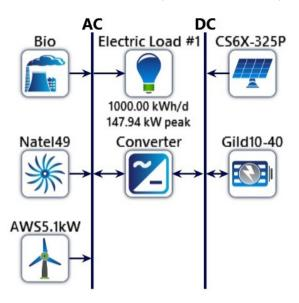
Figure 1. The microgrid power system model for Arusha, Tanzania developed in HOMER Pro<sup>[39]</sup>.
