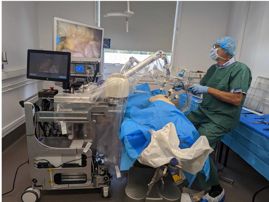
**Figure 3.** The Maestro robotic platform enabling the surgeon to remain in contact with the patient throughout the entire procedure, an example of a non-console robotic system.
