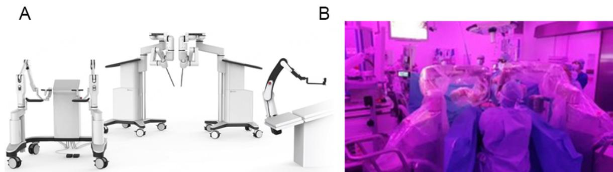
**Figure 2.** (A) The Dexter Complete Surgical System utilizing laparoscopic instruments. (B) an example of a console robotic system enabling the operating surgeon to remain sterile during surgery so that rapid and continual contact with the patient can be maintained throughout the entire procedure. (<https://otjonline.com/featured-articles/distalmotion-dexter/>)
