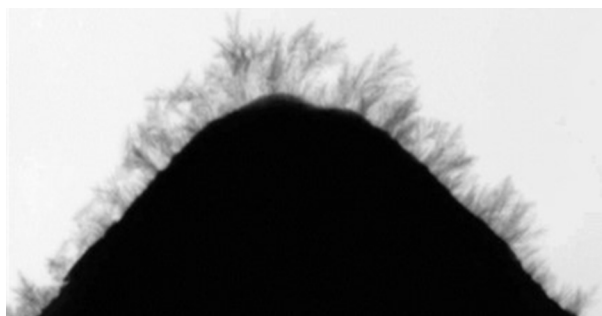
Figure 3. Dendrites on a zinc electrode [16] .
